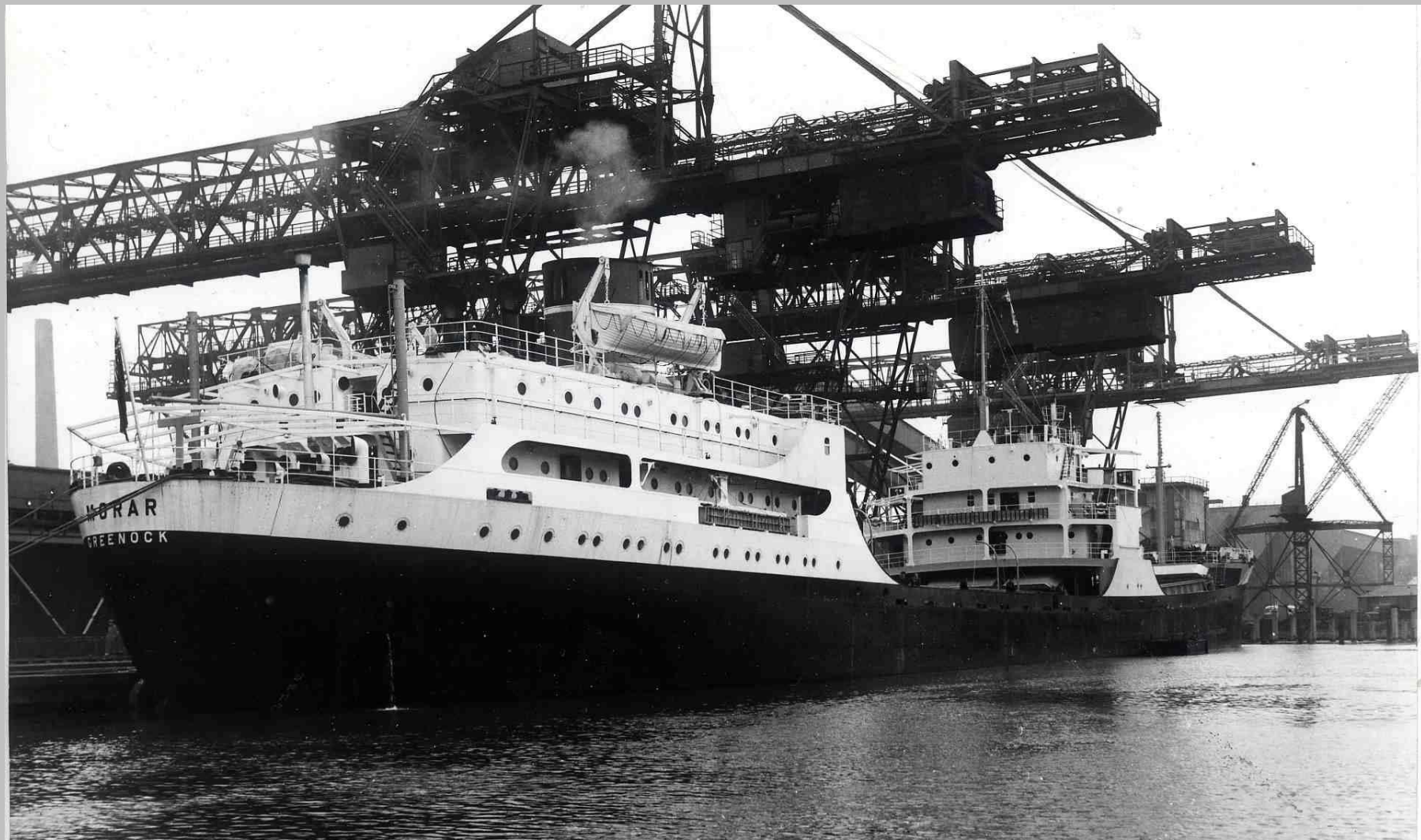
'Morar' Margam Wharf 1956 Powered by experimental free piston Gas Generators. Later sold to a German Company & Re-Engineed with diesel power and renamed mv 'Arnis'. She was scrapped in Taiwan in 1980
